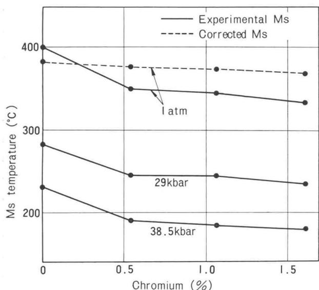
Fig. 1. The Ms temperature in Fe-C-Cr alloys under various pressures. The broken line shows the Ms of Fe-C-Cr alloys at 1 atm corrected at the carbon level of 0.3% C by the Steven's equation<sup>19)</sup>.
